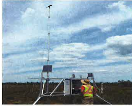
Wainfleet Bog Weather Station for fire index monitoring at the site, as well as additional data for flood forecasting across the watershed and Ontario
