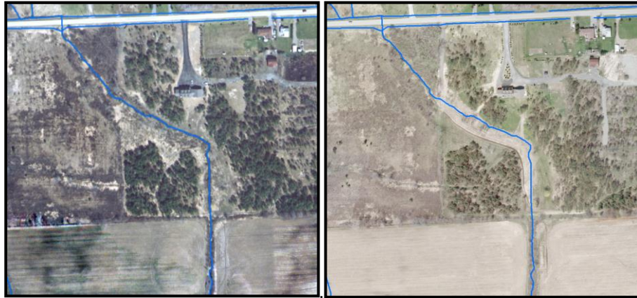
Figure 4: Hydrology breakline feature captured in 2002 (left) not updated to reflect positioning in 2006 photos (right).
