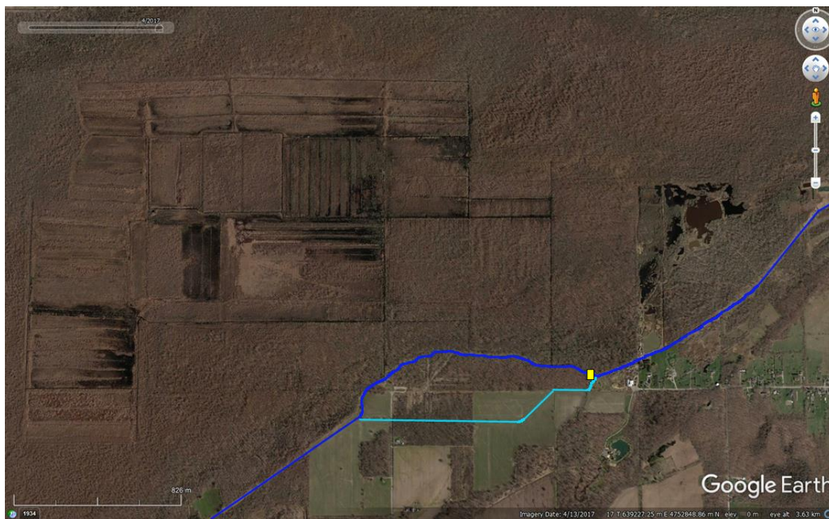
Figure 10. Aerial view of southern edge of Wainfleet Bog, with the current route of Biederman drain in dark blue, and the historical, proposed route in light blue. Yellow rectangle indicates the proposed location of the dam structure to be installed (a one-control-point solution).
