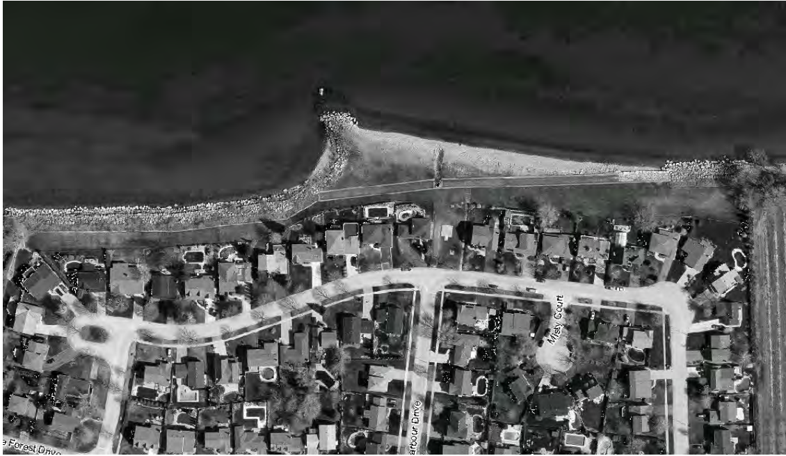
Figure 6.18 Headland Anchored Beach and Revetment (Bal Harbour, Reach 8)
