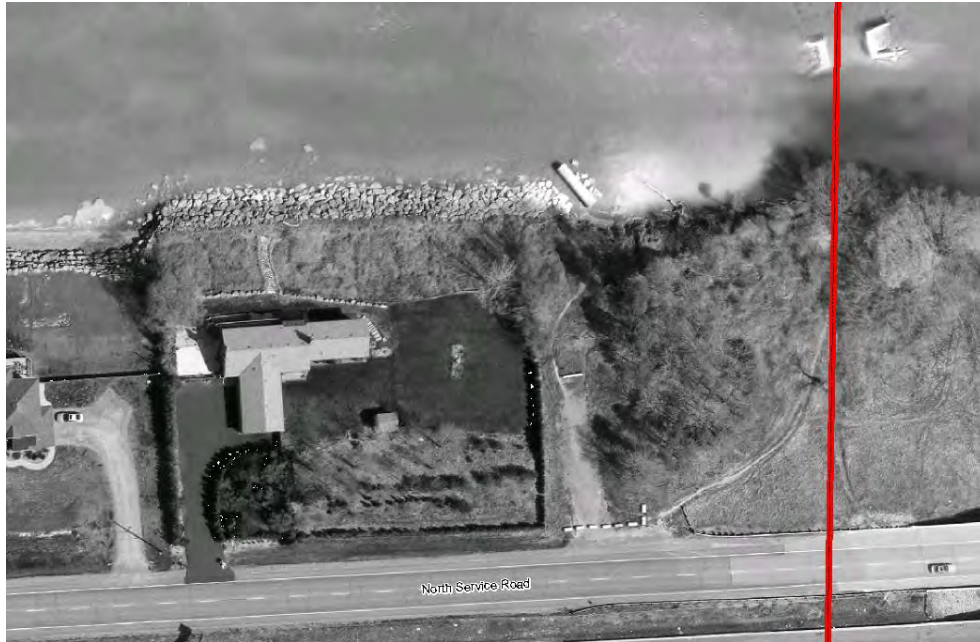
Figure 6.24 Outflanking of Shoreline Protection (right hand side; 13 th Street Road Allowance)
