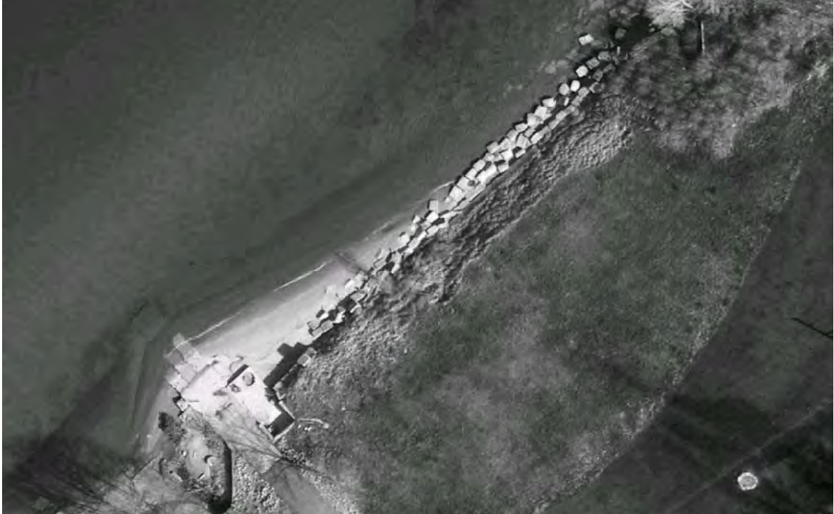
Figure 6.12 Concrete Blocks Appear to Be Toppled (Reach 26, 2006 aerial)
