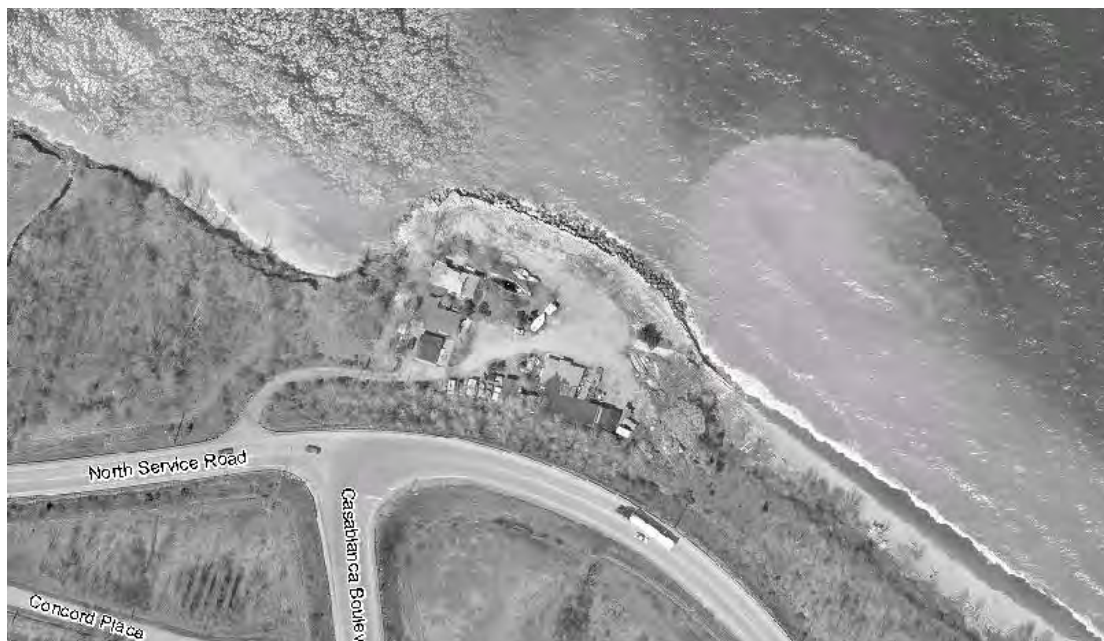
Figure 6.23 Outflanking of Shoreline Protection (left hand side; Reach 2 at Casablanca Blvd.)
