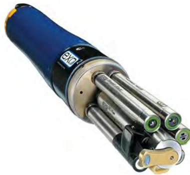
Figure 21. YSI EXO Sensor used at Lake Niapenco
