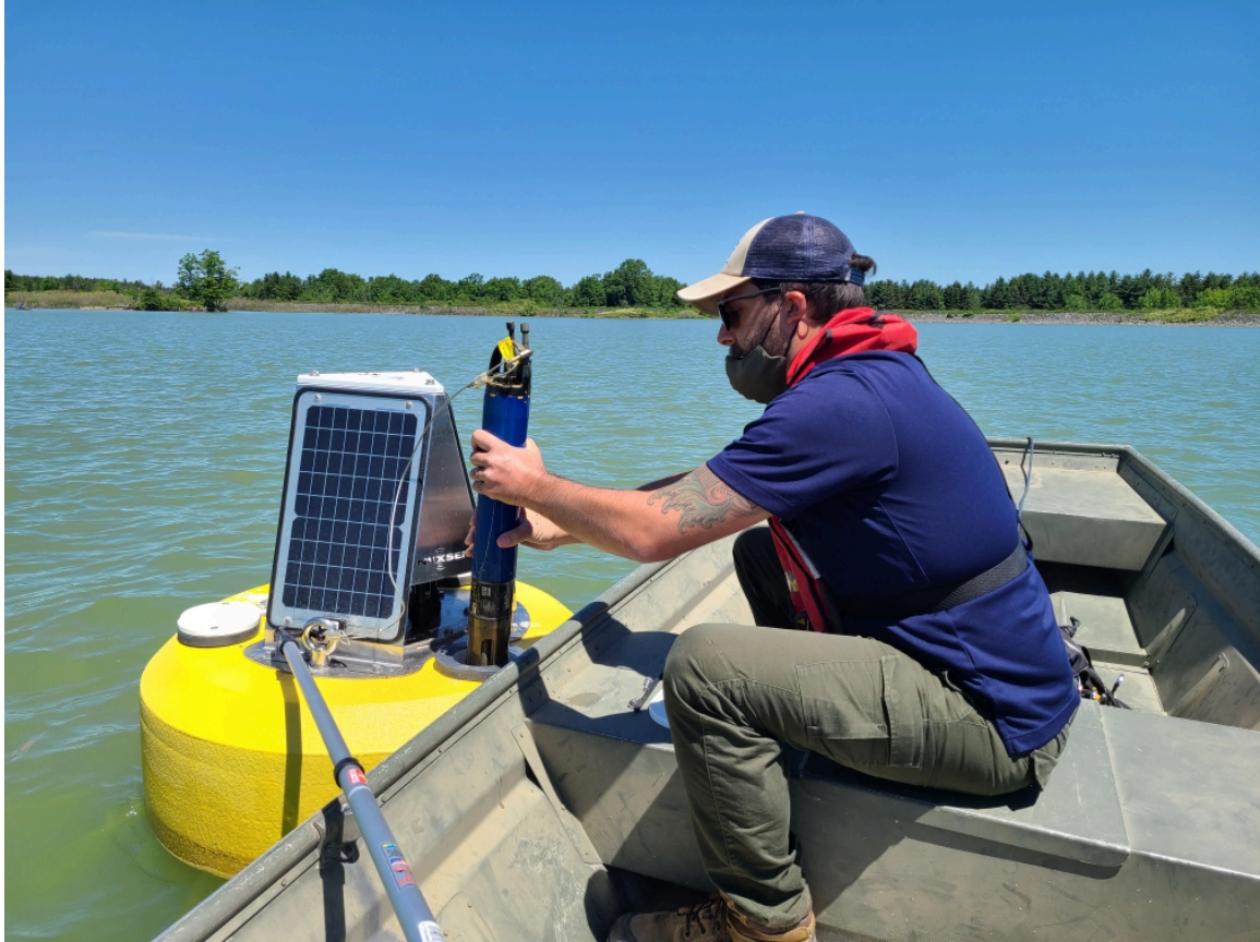
Figure 18: NPCA staff installing an EXO multiparameter sonde in a buoy.
