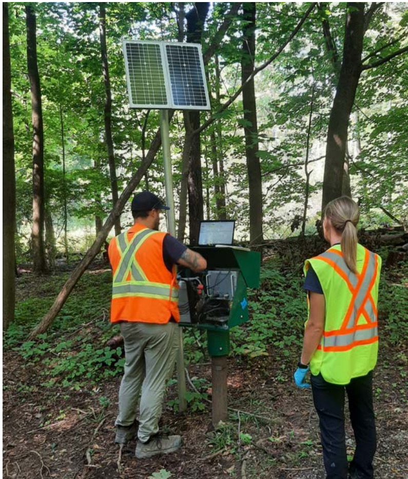
Figure 13: NPCA staff performing routine monitoring on a groundwater well.
